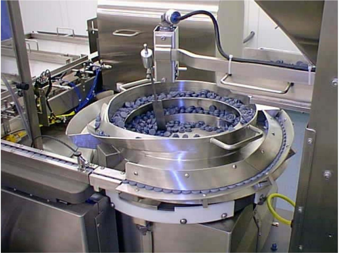
Vibratory stopper bowl is used to orient vial stoppers so that they can be fed into automated placement equipment.
