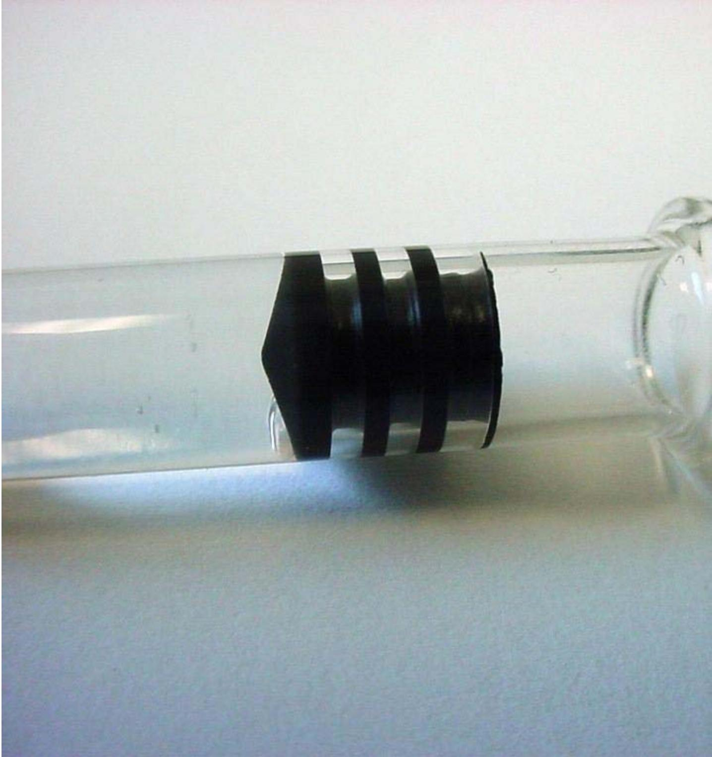
Pre-filled syringe, showing plunger and associated rings. The rings are clear of fluid, which would cause a rejected unit. There
